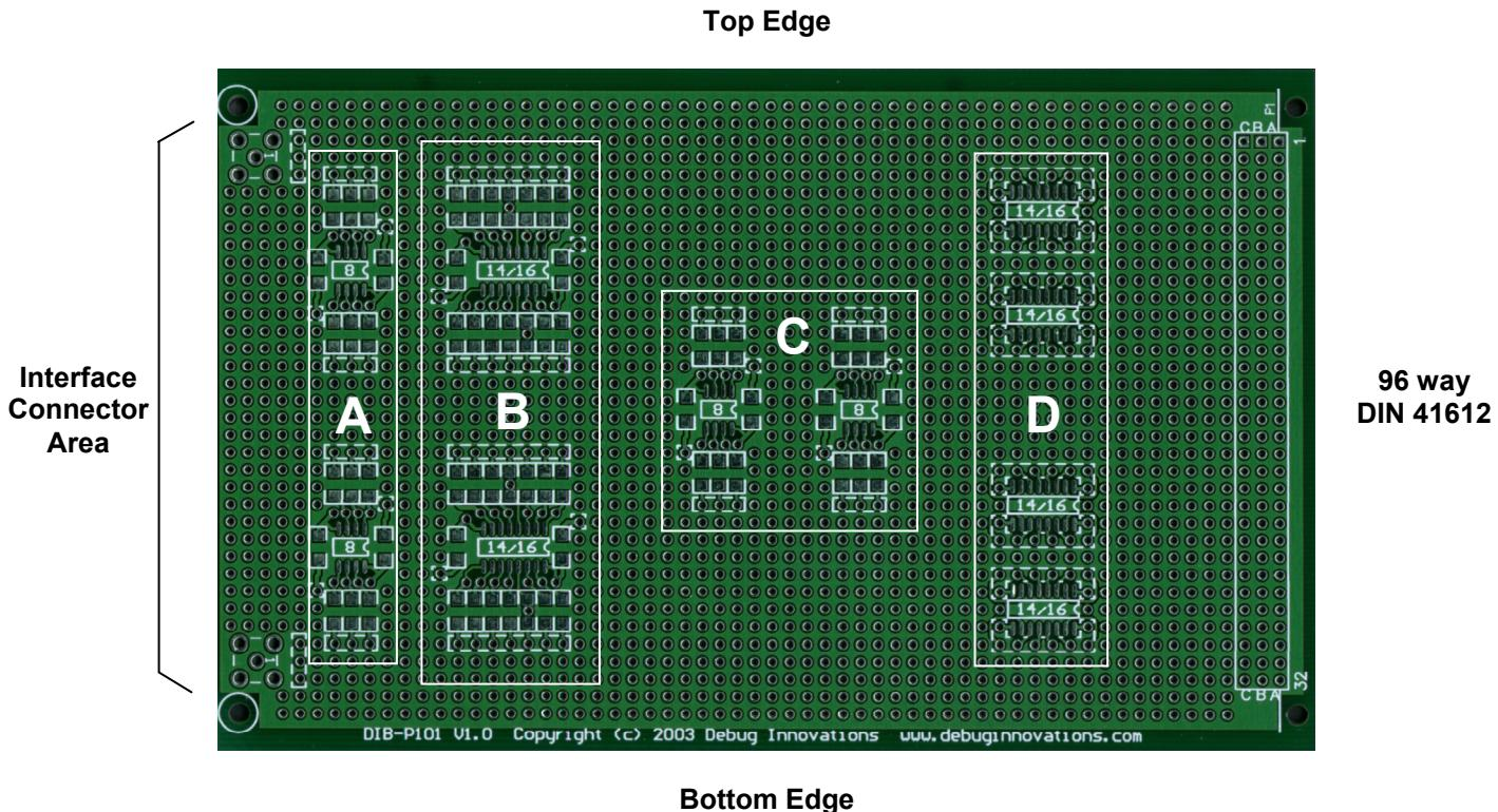
The photo above shows the component side of a DIB-P101 prototype board. The main features are clearly marked. They are:
