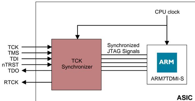
A TCK synchronizer is required to interface synthesizable ARM cores to standard JTAG compliant products such as ICES and production test equipment.
