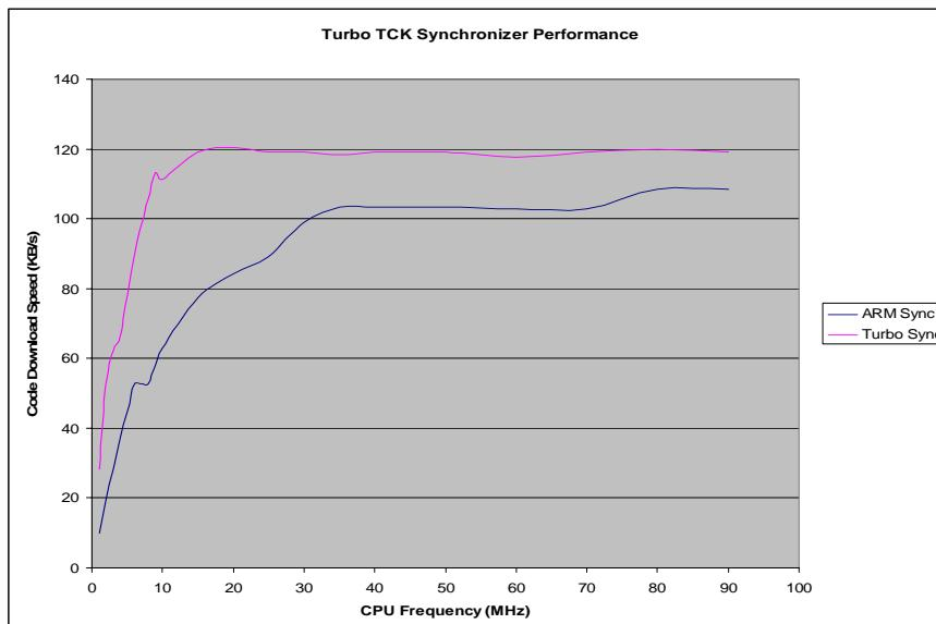
At low CPU clock frequencies, the performance of the Turbo TCK Synchronizer is 3 times that of ARM's standard circuit, at 10MHz the performance is double and above 15MHz the full speed of the ICE is reached (faster ICEs and test equipment would take further advantage of the Turbo Synchronizer's performance) whereas ARM's standard synchronizer doesn't achieve full performance even at 90MHz.
